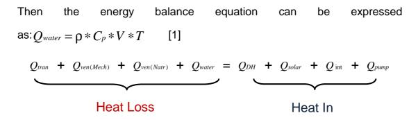
Now we can make the energy survey for each parameter of this equation. It is a clear and efficiency way to analyze the energy balance of the whole building.
