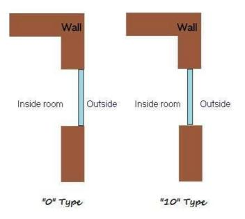
Figure 13: The two types of windows' position
