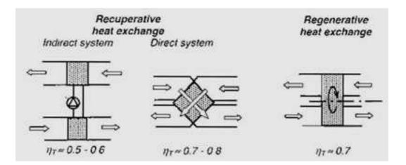
Figure 11: Classification of Heat Exchangers
